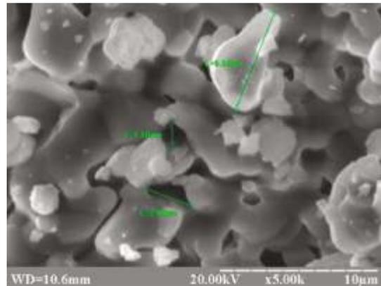
**Fig. 1: Microstructure of the Osteoplastic Material Calc-I-Oss<sup>®</sup>. Mineral Crystals Measuring 6.59 Microns and Micropores between them Ranging in Size from 1, 5 to 2, 89 Microns. Electronic Scanning Image X 5000**
